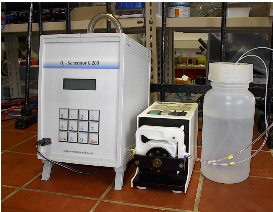
Figure: Oxygen generator with pump device and storage bottle.
