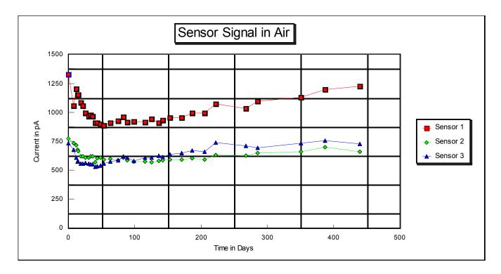
3 sensors are working 24 hours per day on air (room temperature, air pressure) since August 2003 without any maintenance, membrane exchange or electrolyte refilling. The raw data are not temperature and pressure compensated. The test has not been finished yet.
