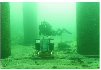
This prototype of an underwater fuel cell system was tested for 8 weeks in the Baltic Sea near the German coast in order to demonstrate the working principle as a first step. For this purpose a small system was selected with low output power and small fuel and oxidant amounts. At the moment there are some further improvements in development like more cells, the extension of the electrode surface and other fuels.
