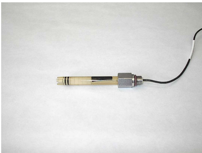
Fig.: pH-combined sensor, shallow water version, OEM-version for integration in probe bottoms
