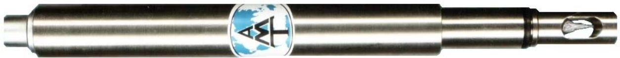
Fig.: Amperometric H 2 O 2 -Micro-sensor, complete with titanium housing, integrated electronics and exchangeable sensor tip
